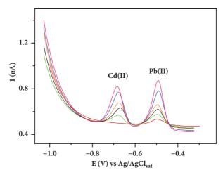
FIGURE 6: Differential pulse anodic stripping voltammograms for 1.00 mL wastewater sample in 9.00 mL acetate buffer solution (pH 4.5) with increasing Cd(II) and Pb(II) concentrations (48.3 to 233  $\mu$ g L<sup>-1</sup>) using BiFE.
