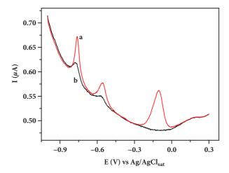
Figure 3: Differential pulse anodic stripping voltammograms obtained for Cd(II) and Pb(II) in 0.10 mol L<sup>-1</sup> acetate buffer solution (pH 4.5) as supporting electrolyte; (a) 250 mg L<sup>-1</sup> of Bi(III) dissolved in supporting electrolyte, (b) without Bi(III), determined with GE containing 142  $\mu$ g L<sup>-1</sup> of Cd(II) and Pb(II) ( $E_{dp}$  = -1.40 V;  $t_{dp}$  = 250 s; potential step =1.95 mV; amplitude = 25 mV).
