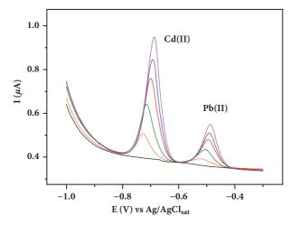
FIGURE 5: Differential pulse anodic stripping voltammograms for increasing concentrations (ranging from 48.3 to 233  $\mu$ g L<sup>-1</sup>) of Cd(II) and Pb(II) in 0.10 mol L<sup>-1</sup> acetate buffer solution (pH 4.5) as supporting electrolyte using BiFE.
