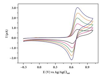
FIGURE 2: Cyclic voltammograms of potassium ferroferricyanide in 2.0 mol L<sup>-1</sup> H<sub>2</sub>SO<sub>4</sub> using GE (scan rate: 100 mV s<sup>-1</sup>).
