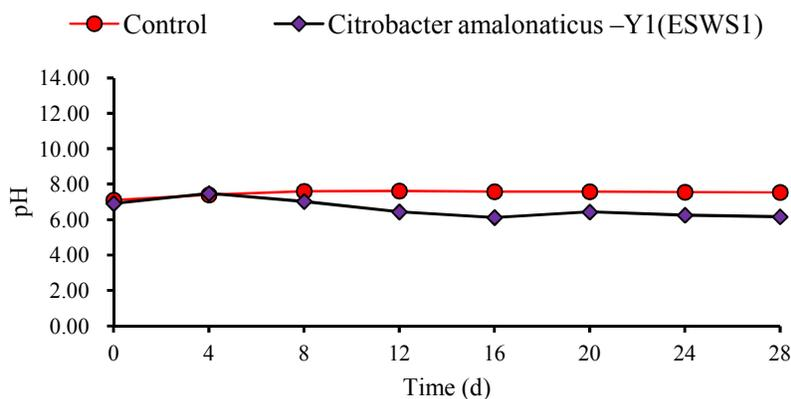
Fig. 1a. Changes in pH during biodegradation of Bonny light crude oil by bacterial isolates obtained from IKO estuarine water ecosystem
