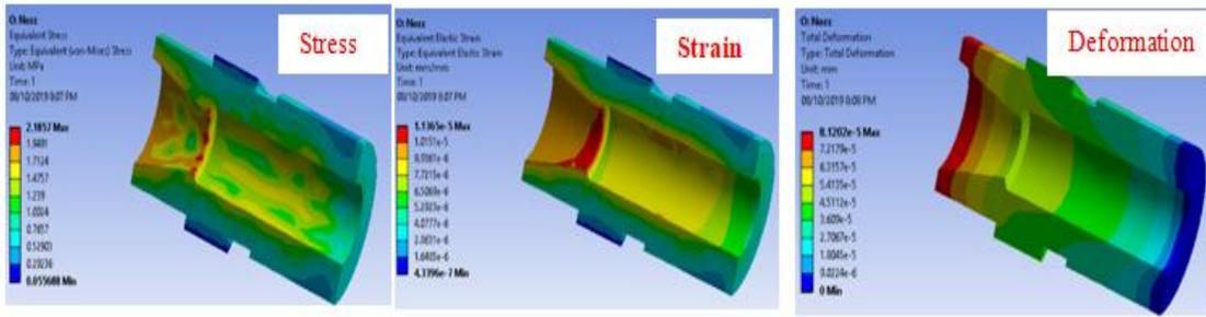
Fig. 3. Values of the stress, strain and deformation of stainless steel Nozzle
