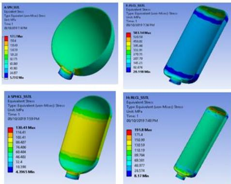
Fig. 2a. Stress analysis of stainless steel
