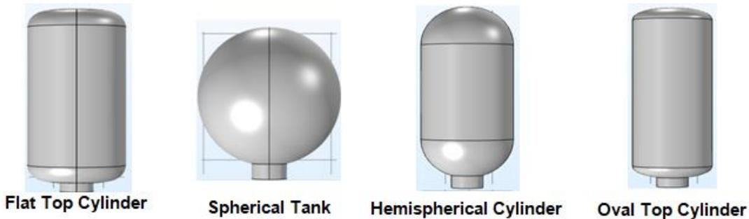
**Fig. 1. Shows the three dimensional renderings of the 4 different geometries of tank**
