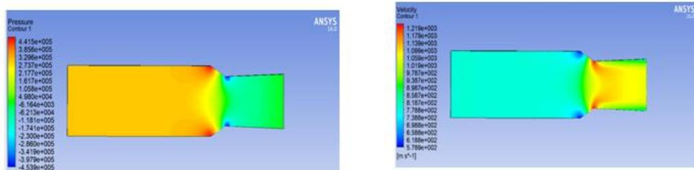
Fig. 4. Pressure contour of the nozzle
