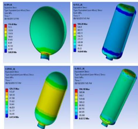
Fig. 2c. Stress analysis of aluminum
