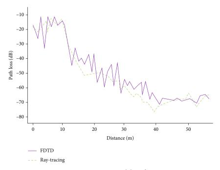
FIGURE 8: Propagation path loss of A-B.
